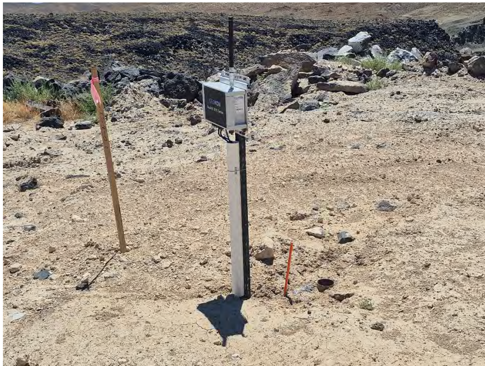
Photograph No. 12.15: 2026 Metallurgical Drill Hole Collar with Piezometer
