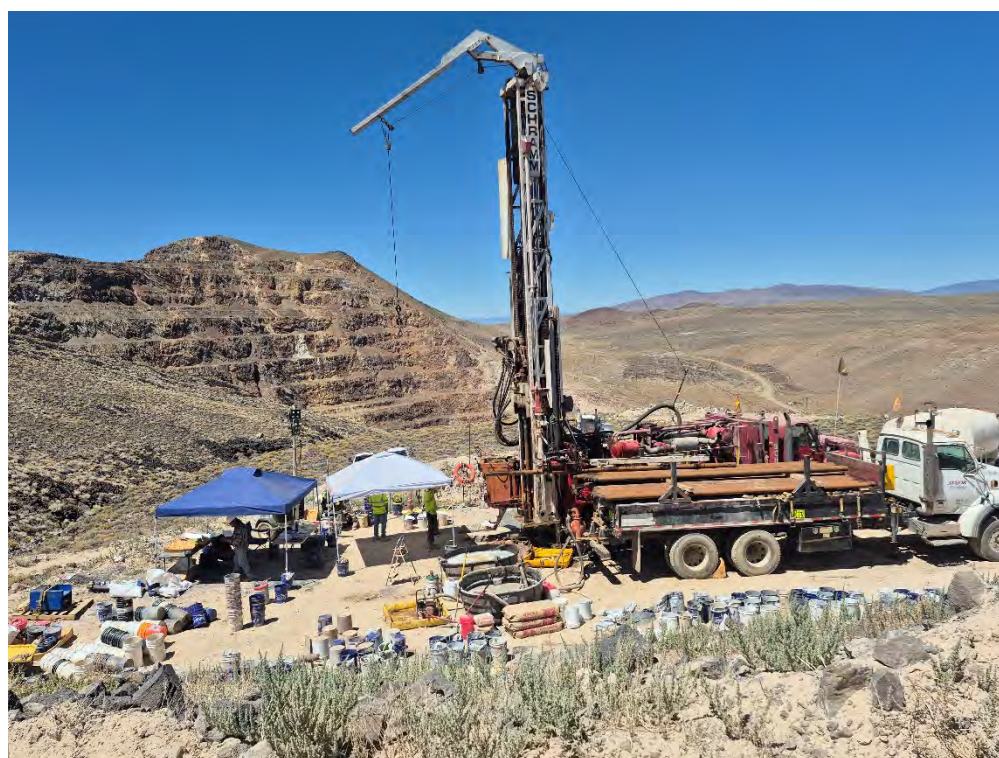
Photograph No. 12.18: 2026 RC Drill Collar with RC Drill
