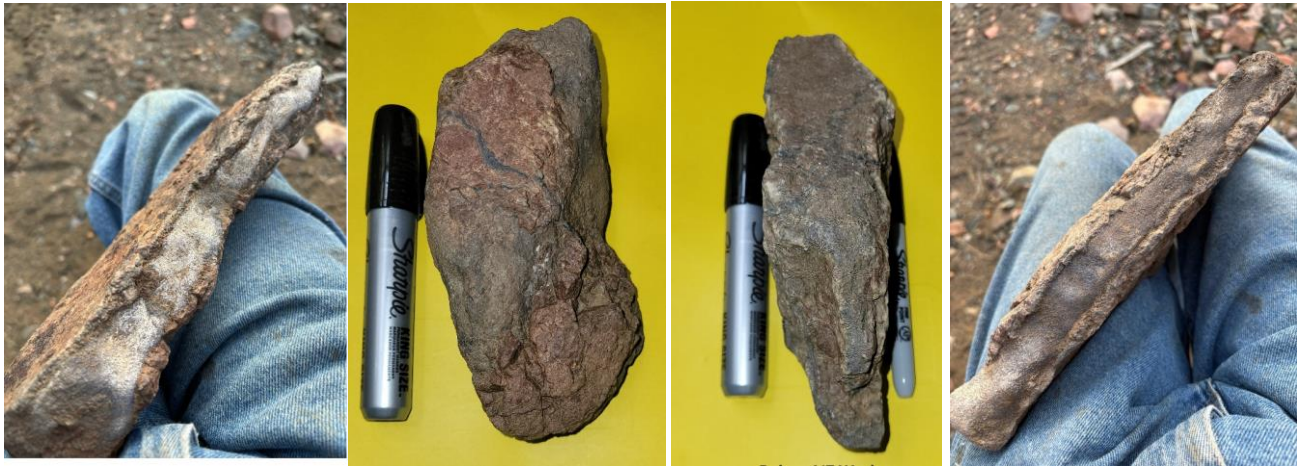
Figure 1. From left to right: 5 lb silver fragment with quartz walls, 4.7 lb silver fragment (70% native silver) with dark gray coating of cerargyrite and a patch of hematized quartz, 3.4 lb silver fragment (45% native silver) with hematized quartz matrix and white quartz walls, 6.2 lb silver vein fragment with white quartz walls. See Figure 2 for location. Estimated silver contents are based on specific gravity calculations.
